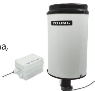
Merilnik padavin (vir: thethingsnetwork.org)
